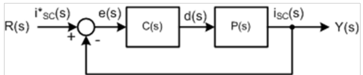
Figure 5.7: Closed loop current control Block Diagram
