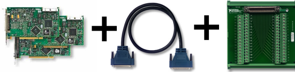
Figure 3.7: Voltage Measurement Hardware
