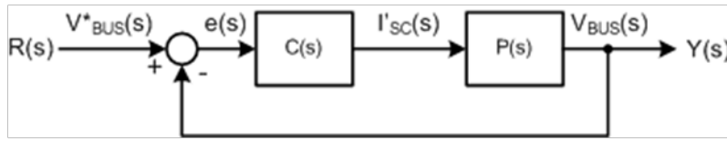
Figure 5.18: Voltage Closed-Loop Block Diagram
